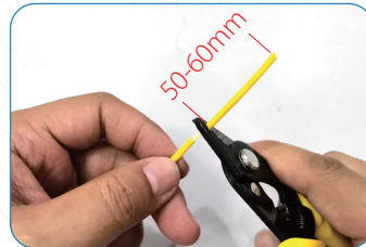
2.2 Strip the cable strengthen layer
