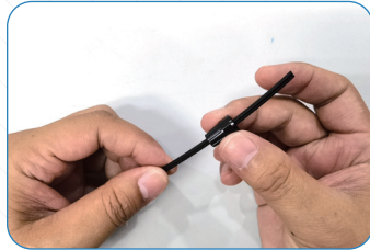
2.1 Put the cable into the boot
