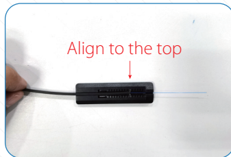
2.6 Put the cable into the cutting clamp
