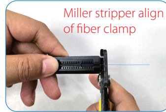
2.3 Press the cable into the clamp
