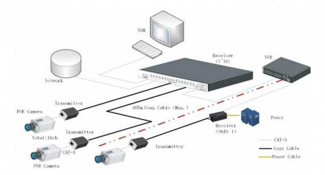
• Application 1: 1ch EoC transmitter VEC11T-EC + 16ch EoC receiver VEC116R-PC. As shown on the left of the red dotted line, a maximum of 16 transmitters may be connected to the receiver.
